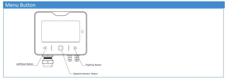
The menu can be navigated using 3 buttons located on the display bezel. The CENTER button is used for selecting the menu item or incrementing the value. The LEFT button is used to move the cursor in the left direction or move down through the menu items. The RIGHT button is used to move the cursor in the right direction or move up through the menu items.
